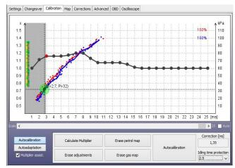
If everything has been installed properly, 4 steps mentioned above should guarantee proper driving on both fuels. In more sophisticated cars there may be necessity of using features located in "Map", "Corrections", Advanced" and "OBD" bookmarks. To learn more details refer to the User's Manual located in "docs" folder attached to the software (Press "Help" bookmark to open that folder).
